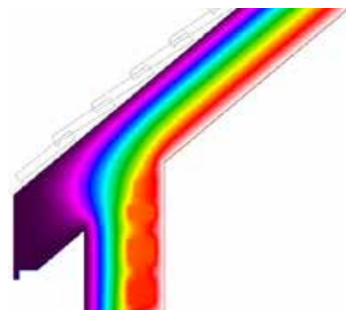
The illustration presents very good thermal protection ensured by the use of the MP element while constructing the knee wall. Continuity of the insulation layer protects the building from heat loss and moisture.
