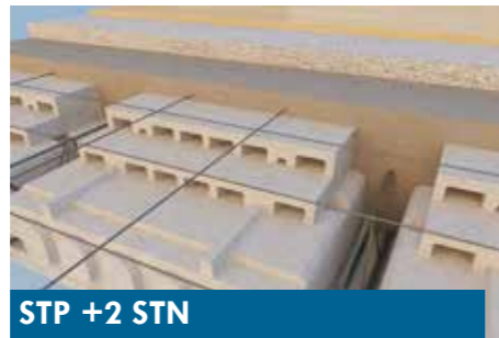
STP Span: < 5.5 m, height: 25 cm Concrete consumption: 70 l/m 2
